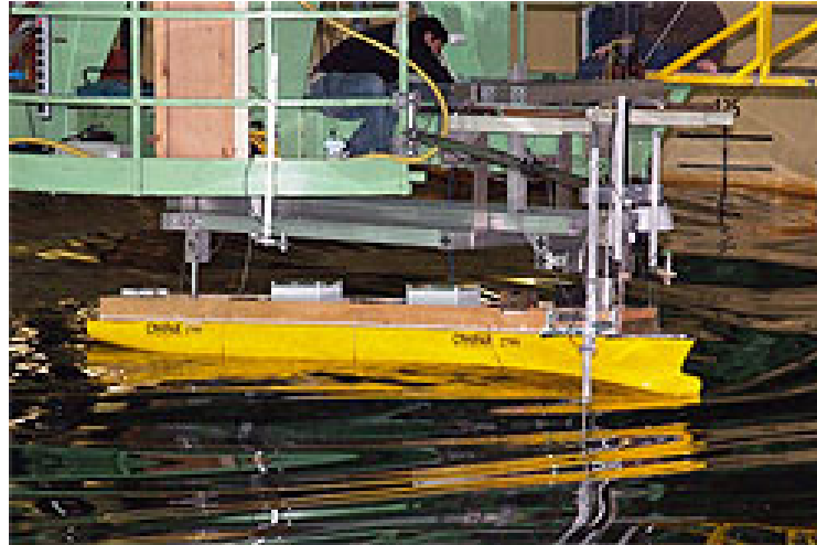
Figure 6-3. Experimental setup for the parametric rolling tests
